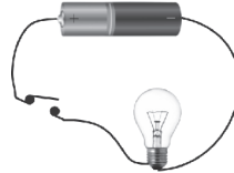
Open circuit (The bulb does not glow.)
